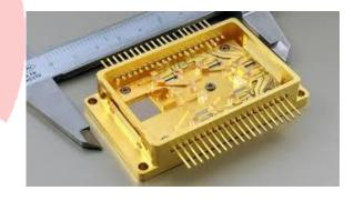
Photonics components to be actively aligned in a package/substrate Lens, prism, filter, optical fiber, ferule, FAC, fiber array...
